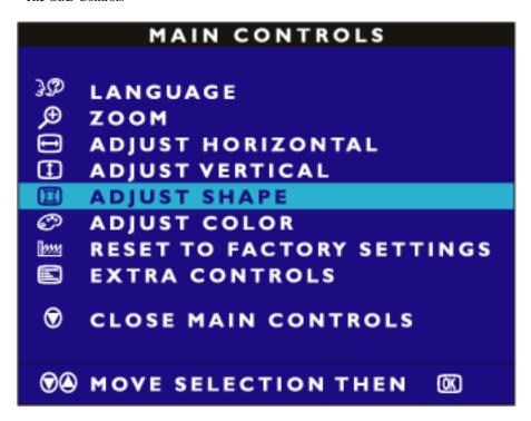
3) Press the **log** button. The ADJUST SHAPE window appears. ADJUST SIDE CURVE should be highlighted.
